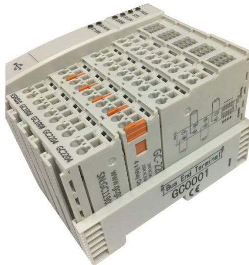
Figure 2.4 GC-0001 Terminal resistance module installation method
