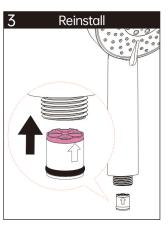
Default restrictor in North America is 1.75 gpm, compliant with California Energy Commission (CEC) regulations. Please check your local plumbing codes before removing it or replacing it with other check valves.
