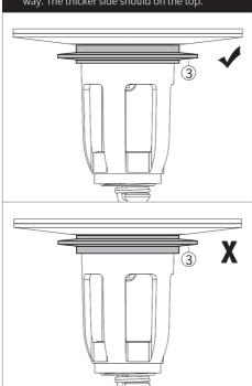
5 After putting the rubber ring in place, put the drain plug over the sink hole and push it down gently to finish the installation.
